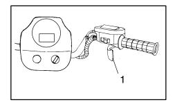
a frozen or stuck throttle. In the event the throttle cable should stick in an open position, the engine will stop and power to the rear wheels will cease when the operator releases the throttle lever.
